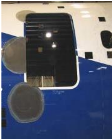
Component test article with SRM-type repairs
