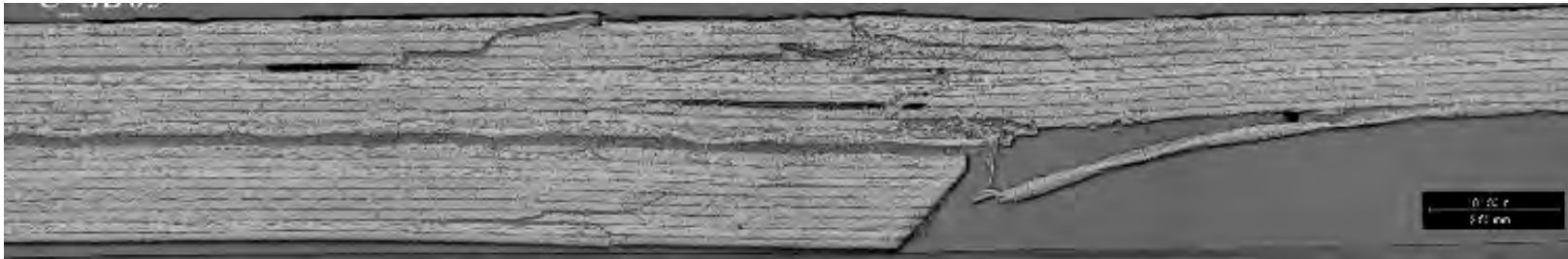
Cross-Section of BVID at a Skin-to-Flange
