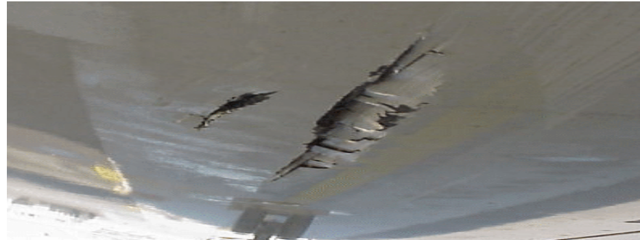
Accidental Damage to Lower Fuselage
